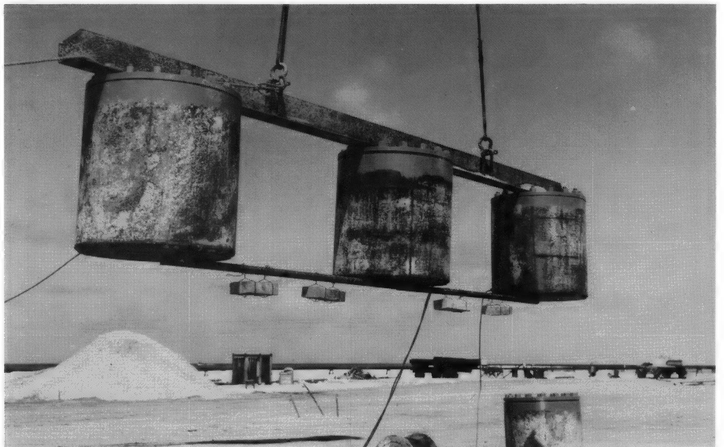
FIGURE 9-13b. HARDTACK, SHOT CACTUS, LOWERING DRUM GAUGES, TAKEN 28 MARCH 1958
